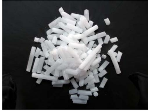
The percentage of sublimation is very low, between 5% to 15% daily, depending on the quality of the container and the environmental conditions. The use of specially insulated containers of approved specifications and certified for dry ice use will keep the rate of sublimation within the above range. Otherwise, if the container is not suitable, the rate of sublimation will be higher. MICHAEL TSONTOS S.A provides all the necessary equipment that is required for the right and safe use of dry ice.
