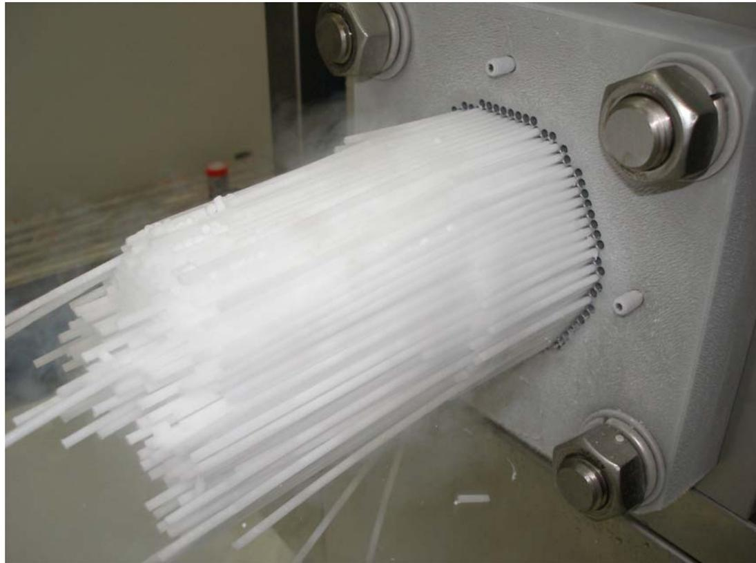
The device that compresses the dry ice into pellets is called pelletizer. After the production, the pellets are placed in specially insulated containers for storage until they are used for the various applications.
